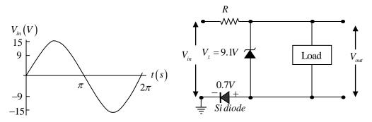
The forward voltage drop for silicon diode is 0.7 V and the Zener voltage is 9.10 V. If the input voltage  $(V_{in})$  is sine wave with an amplitude of 15 V (as shown in the figure above), which of the following waveform qualitatively describes the output voltage  $(V_{out})$  across the load?
